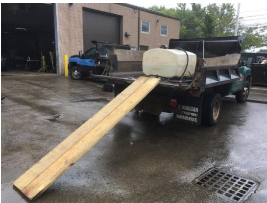
Figure 5 – Dump truck with wood planks set up as a ramp
